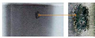
**Electric arc pitting:** Burns created by improper electric grounding while bearing is stationary.
