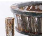
**Etching:** Rusting with pitting and corrosion from moisture.
