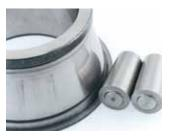
**Abrasive wear:** Fine abrasive particle contamination.
