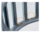
**Cage pocket wear:** Heavy contact between rollers and cage pocket surfaces caused by bearing operating too loosely.
