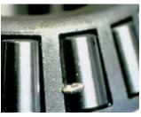
**Grooving:** Large particle contamination embedding into soft cage material.
