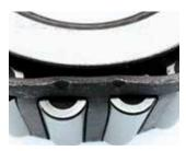
**Cage deformation:** Improperly installed or dropped bearing.
