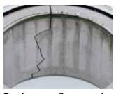
Bearing cone (inner race) bore damage: Fractured cone due to out-of-round or oversized shaft.
