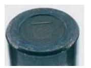
**Bearing cone (inner race) large rib face scoring:** 'Welding' and heat damage from metal-to-metal contact.
