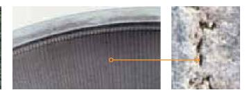
**Fluting:** Series of axial burns caused by electric current passing through the bearing while rotating.
