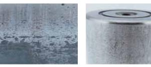
**Micro-spalling:** due to thin lubricant film from high loads and low RPM or elevated temperatures.
