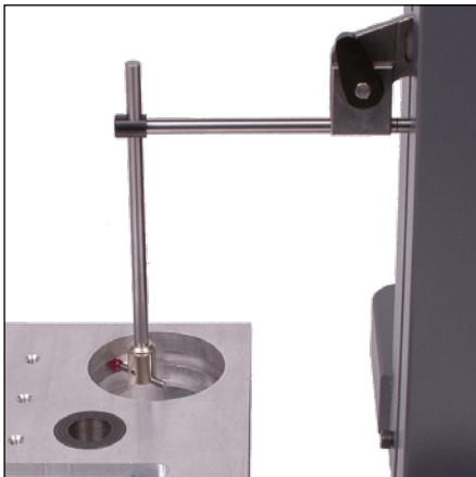
Internal groove measurement with accessories 930.2108, 930.2110 and 905.2207
