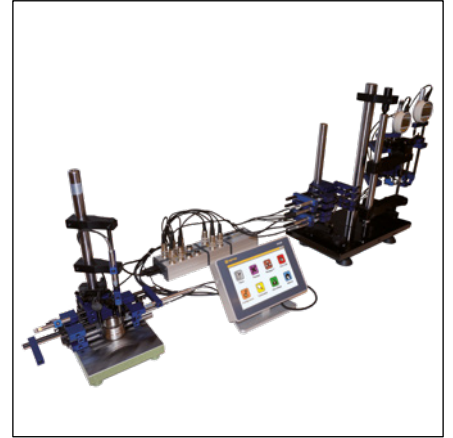
Probes and indicators connection through M-BUS inputs
