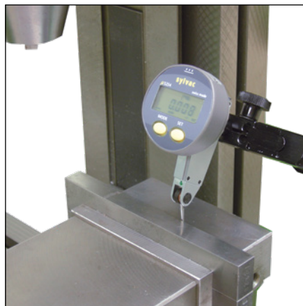
Checking the alignment on milling machine.
