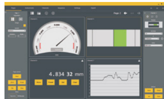
Multi-channel display with colour-coded tolerances
