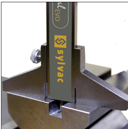
Depth measurement with S_Cal EVO and base 910.2205.
