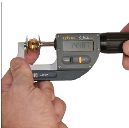
Part measurement with a S_Mike PRO Disk
