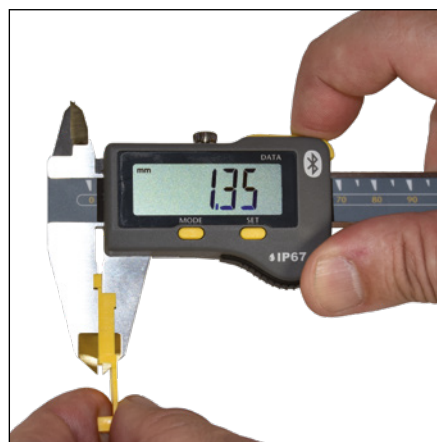
Part measurement with sending data
