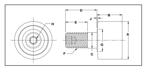
Plain Track Rollers effectively carry radial loads. For heavy side loads, they can also be positioned to act as side guides.
