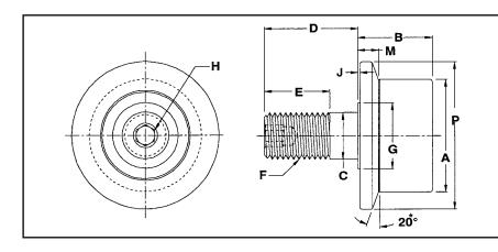
Flanged Track Rollers are used where light side thrust loads exist. When used in this manner, the flange acts as a guide. Flanged Track Rollers are also used in combination with Plain Track Rollers.
