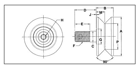
V-Grooved Track Rollers are designed to operate on "V" bar tracks, common in environments where sand, powder or chips would be likely to build up on a flat track.
