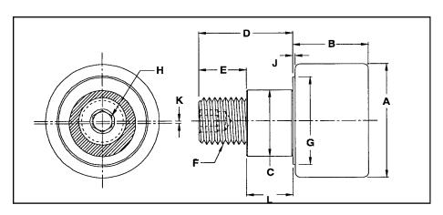
Eccentric Track Rollers are used where precision alignment is necessary. The stud can be rotated before the roller is tightened into position, which overcomes locational tolerance and unequal loading of multiple rollers. It will also help with alignment in guiding applications.
