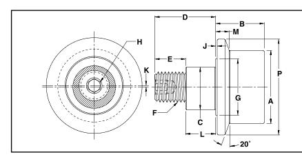
Flanged Eccentric Track Rollers are used where precision alignment is necessary. The stud can be rotated before the roller is tightened into position, which overcomes locational tolerance and unequal loading of multiple rollers. It will also help with alignment in guiding applications.
