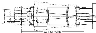
Recommended maximum swivel angle on each side of the cylinder centerline.
