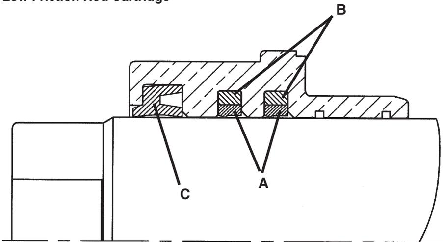
**A** - Dual step-seal rod seals insure positive sealing and smooth operation up to 2,000 PSI.
