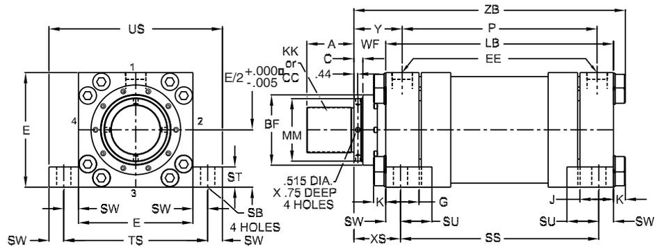
**Note:** Stroke lengths on lug mounted cylinders should not be shorter than the cylinder bore diameter. Consult factory for recommendations on shorter stroke lengths.
