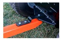
**VERSATILE** Universal hitch can be attached to most tractor drawbars.
