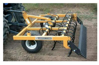
Equipped with 8" wide flotation wheels. Quick hitch compatible.
