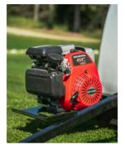
Powered by 5 HP Honda Gas Engine.
